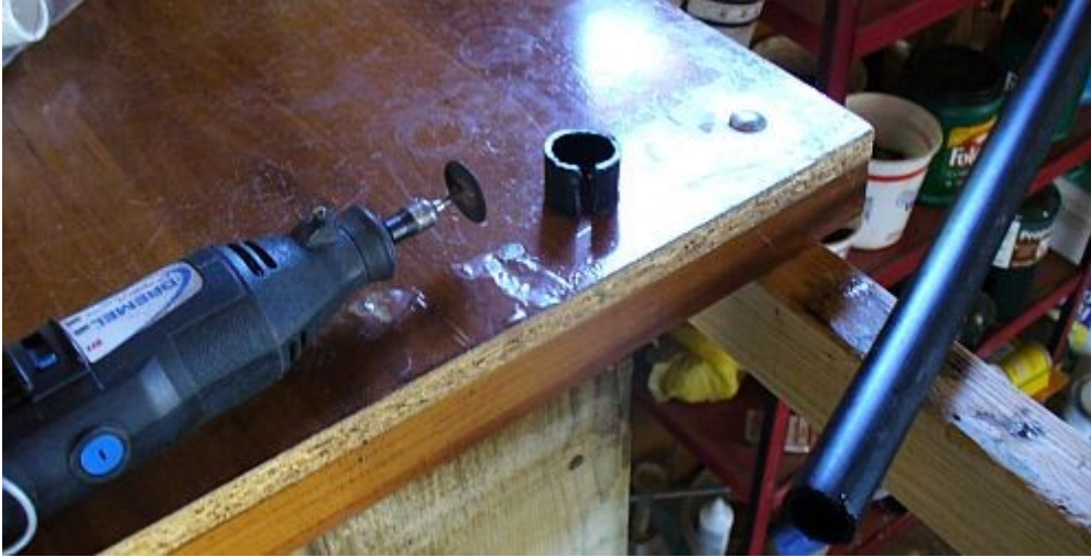
Cut bushing with moto-tool
