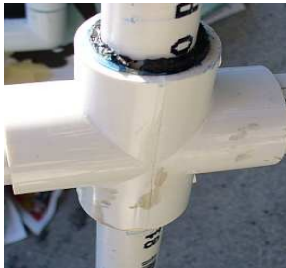
Slider on a vertical support with one of the bushings showing
