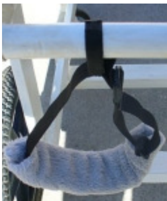
Strap with plastic buckle made from webbing covered with fleece. Overlapping Velcro is used to attach the strap to the bar.
