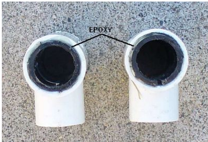
Bushings epoxied in place
