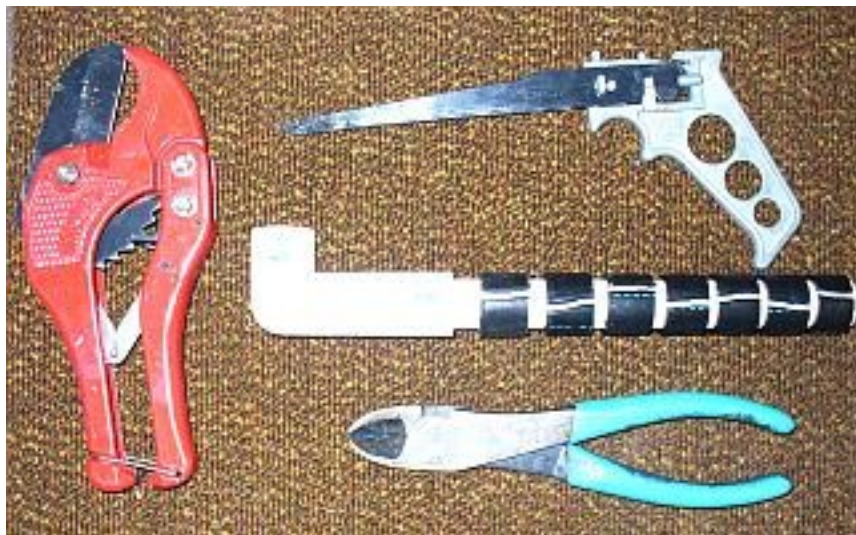
Cut bushings on pipe with other cutting tools
