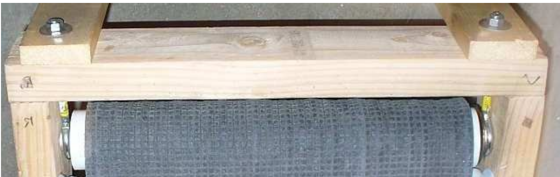
Top view of eye hook placement for the upper roller
