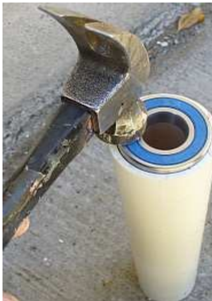
Checking bearing for fit
