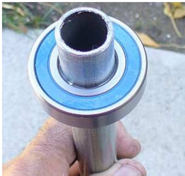
Bearing placed on EMT pipe
